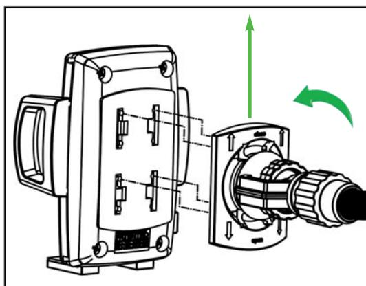
Insert the four hooks of the locking plate into the smartphone holder and push the locking plate in the direction of the arrow CLOSE. The smartphone holder audibly clicks into place on the locking plate. If required, the mount of the smartphone holder can be rotated by 180°. This may be necessary if operating elements on the smartphone are covered by the holder. In this case, the support brackets must be mounted in the opposite groove.
