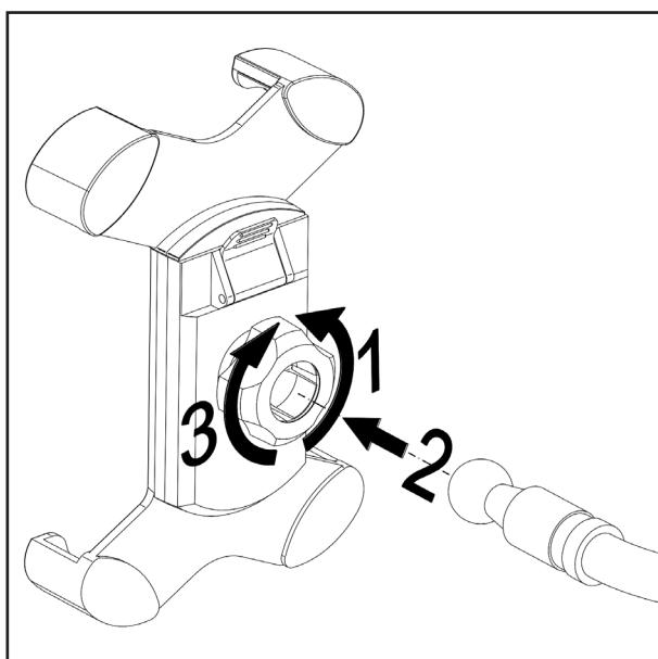
**1** Open the clamping nut on the smartphone holder in the UNLOCK direction until the ball adapter **2** snaps into the smartphone holder with slight pressure.
