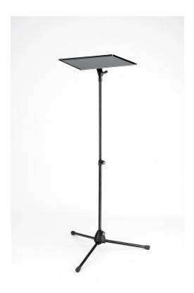
The convenient and comfortably sized laptop rest of 400 x 290 mm is large enough to hold notebooks, laptops or similar products in a range of sizes. The V-shaped connector means the laptop rest can be quickly detached for transport. Its angle can also be altered to any position with the clamping lever. The stable 3-legged base section folds compactly.
