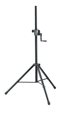
A high quality steel speaker stand with plastic clamps for professional use. Infinitely variable height adjustment with a hand crank and push button system which prevents an uncontrolled reverse motion. There is an additional locking screw for extra safety. Extension tube diameter 35 mm, suitable for speakers and lighting crossbars with an integrated M10 thread connector.
