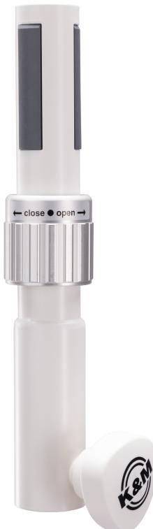
Steel adapter sleeve attaches to speaker stands with tubing diameter of 35 mm, mounts with a locking screw. Integrated unique patented expanding mandrel system which provides a tight and firm fit for the speaker. The moveable plastic splints separate the speaker from the stand creating a vibration-free connection.
