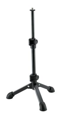
The telescopic microphone stand with a 3/8" threaded connector is extremely versatile. Its height can be adjusted from 230 to 400 mm using the practical clamping lever. This light-weight tripod stand with folding legs is suitable for mobile operation. The robust foot end caps provide stability and reduce undesirable transmission noise.
