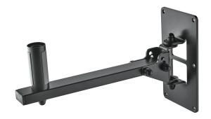
Robust wall mount for holding speakers with flange socket up to 25 kg. The swivel range is continuously adjustable up to 120°. The tilt can be fixed in three steps with 0°, -12.5° and -25°. A patented expanding mandrel ensures a wobble- and vibration-free fit of the speaker. The solid steel construction and durable powder coating ensure long-lasting use.
