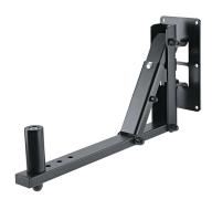
Robust speaker wall mount for speaker cabinets with flange socket receptacle. Max. recommended load 25 kg. Thanks to the appropriate design, the bracket is almost completely concealed by the speaker. The speaker distance to the wall is selectable in 4 steps. The swivel range is infinitely adjustable, and the tilt angle can be fixed in 6 steps up to max. 30 °.
