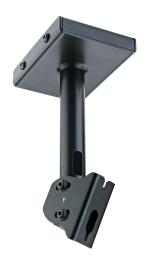
Robust and useful loudspeaker ceiling mount with 250 mm distance and internal cable management. The swivel area is +/-45 °. Within the parameters - the settings range from 0 to 45°. The clamping bracket is for loudspeakers with a vertical mounting template from 70 to 76.2 mm. For other attachment possibilities additional adapter brackets are available. A mounting bracket with side and central cable management makes mounting to the ceiling easier.
