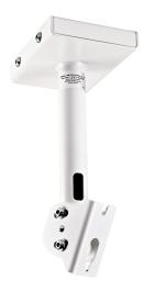
Robust and useful loudspeaker ceiling mount with 250 mm distance and internal cable management. The swivel area is +/-45 °. Within the parameters - the settings range from 0 to 45°. The clamping bracket is for loudspeakers with a vertical mounting template from 70 to 76.2 mm. For other attachment possibilities additional adapter brackets are available. A mounting bracket with side and central cable management makes mounting to the ceiling easier.
