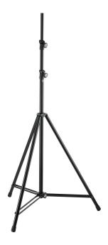
Extending to over 4 m, this lighting stand is for professional use. The new zinc die-cast clamps and the larger steel leg tubing give this top of the range stand more stability. The infinitely variable non-marring height adjustment can be reinforced with two safety rings. A variety of crossbars may be attached using the M10 thread adaptor.
