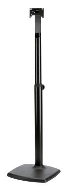
Steel stand for the Genelec 8000 monitor series. This stable elegant stand has a 420 x 420 mm cast base with an oversized rod combination. Gradual height adjustment is made by a superior positioning and clamping knob. Quick, uncomplicated mounting of the monitor is accomplished using the suspension device.
