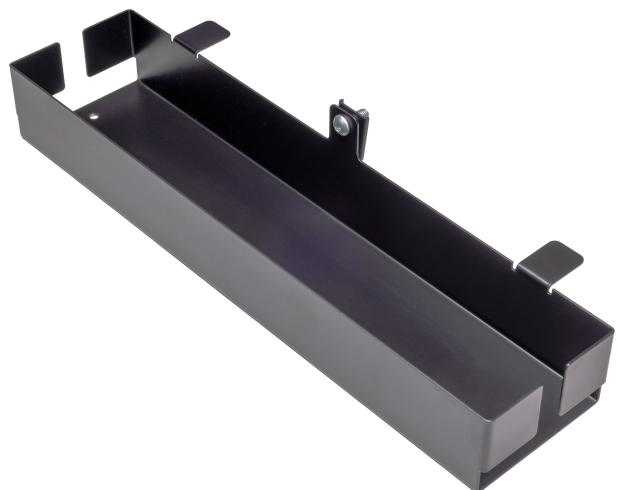
The practical box is attached to the crossbar of the confidence monitor stand close to the ground and is used to hold power strips and neatly store extra-long cables. The solid construction made of sturdy sheet steel has side openings that provide enough space for convenient cable routing. The dimensions are 437 x 100 x 60 mm.
