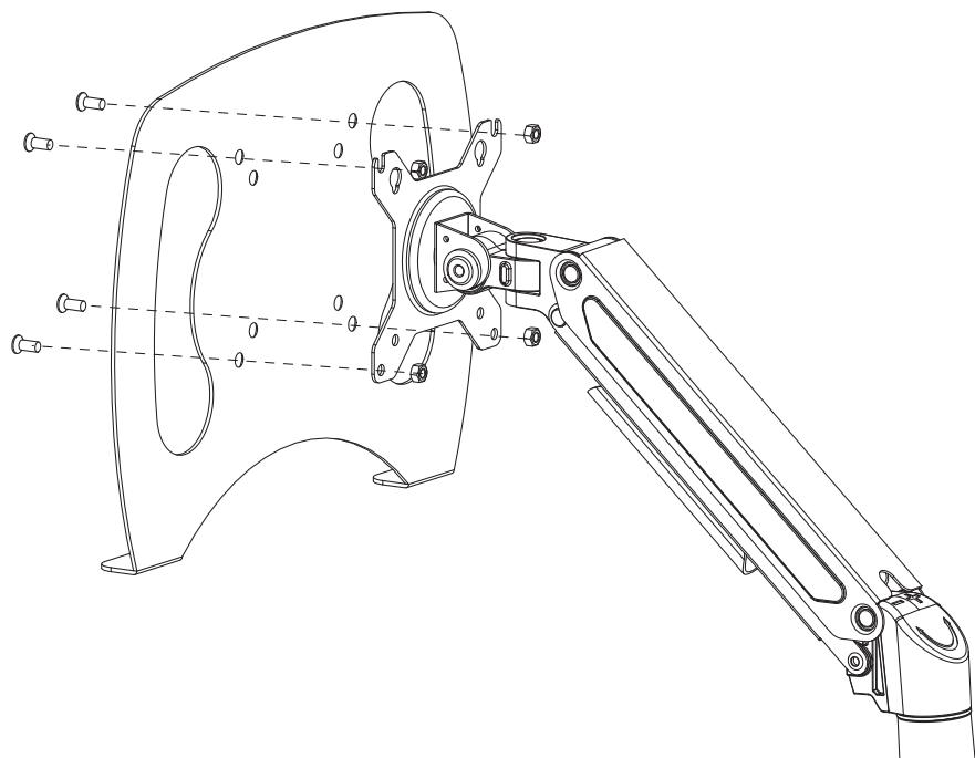
Install the Laptop Tray with screws and nuts included in the package D using 4mm Hex Wrench.
