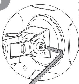
Use a hex wrench to adjust the damp for tilting. Turn counter-clockwise to reduce damping and clockwise to increase damping.
