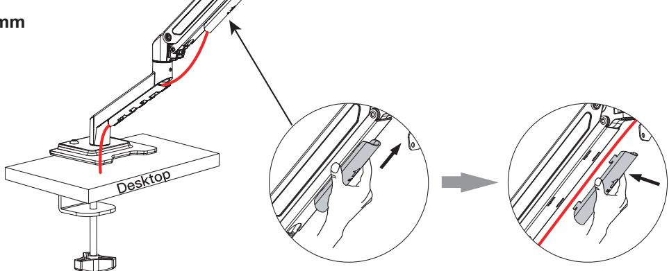
Insert cables into cable covers. Leave enough slack of cables at arm joints for full adjustment.
