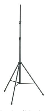
This compact overhead microphone stand is now even lighter and more stable. Thanks to a new leg combination and a new clamping element, its weight has been reduced to 8.37 lbs. The leg base diameter of 39.37 affords stability and safety. A range of different boom arms can be attached using the 3/8" thread adaptor. The stand extends to a height of over 120".
