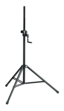
A high quality steel speaker stand with zinc die-cast clamps for professional use. Infinitely variable height adjustment with a hand crank and push button system which prevents an uncontrolled reverse motion. There is an additional locking screw for extra safety. Extension tube diameter 1.378", suitable for speakers and lighting crossbars with an integrated M10 thread connector.
