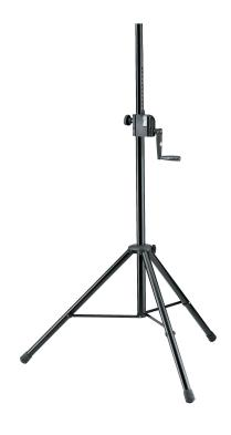
A high quality steel speaker stand with plastic clamps for professional use. Infinitely variable height adjustment with a hand crank and push button system which prevents an uncontrolled reverse motion. There is an additional locking screw for extra safety. Extension tube diameter 1.378", suitable for speakers and lighting crossbars with an integrated M10 thread connector.
