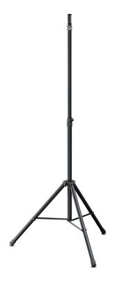
A patented expanding mandrel with quick-release fastener ensures a tight fit of the speaker cabinet. The plastic expansion splints ensure a vibration-free connection between the speaker cabinet and the tube. The height of the steel stand ranges from 55.787 to 83.346", is fixed with a safety hook and secured by a clamping screw for a vibration-free and firm fit. Other features include a pull-out guard for the extension tube, an integrated shock absorber and durable powder coating.
