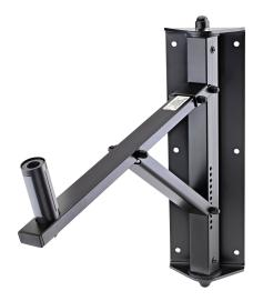
The swivelling and tiltable wall mount holds your speaker at the angle you want. The mount has 11 different tilt settings moving through 22°. The swivel is adjustable to any angle. The patented expanding mandrel for loud speakers with cabinet interiors of diameter from 1.378 to 1.457" is tightened with a key for a non-wobble and low-resonance speaker fit.
