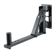
Robust speaker wall mount for speaker cabinets with flange socket receptacle. Max. recommended load 55.066 lbs. Thanks to the appropriate design, the bracket is almost completely concealed by the speaker. The speaker distance to the wall is selectable in 4 steps. The swivel range is infinitely adjustable, and the tilt angle can be fixed in 6 steps up to max. 30 °.
