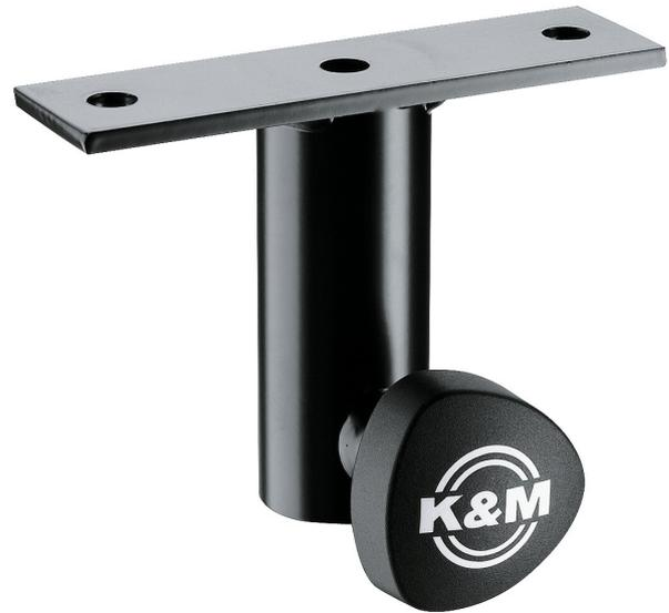
Attachable to speakers. Slip-on adapter for speaker stands with tube-diameter 1.38". With 2 drill holes diam. 0.43" at intervals of 4.53" and locking device. Mounting bolts M10 x 1.574", washers and nuts (2 of each) included.
