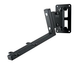
Stable wall mount for JBL loud speakers. The wall mount swivels approx. 60° to the right and to the left. And the mounting plate can also tilt up to 30°. The extension arm is simply screwed to the loud speaker or monitor, which is then attached to the wall mount. Screws and keys are included. The maximum load bearing weight is 44.53 lbs. The mount is suitable for JBL Series LSR 2328 P, 2325 P, 4328 P and 4326 P.
