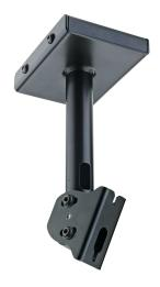
Robust and useful loudspeaker ceiling mount with 9.842" distance and internal cable management. The swivel area is +/-45 °. Within the parameters - the settings range from 0 to 45°. The clamping bracket is for loudspeakers with a vertical mounting template from 2.75 to 3". For other attachment possibilities additional adapter brackets are available. A mounting bracket with side and central cable management makes mounting to the ceiling easier.
