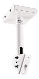
Robust and useful loudspeaker ceiling mount with 9.842" distance and internal cable management. The swivel area is +/-45 °. Within the parameters - the settings range from 0 to 45°. The clamping bracket is for loudspeakers with a vertical mounting template from 2.75 to 3". For other attachment possibilities additional adapter brackets are available. A mounting bracket with side and central cable management makes mounting to the ceiling easier.
