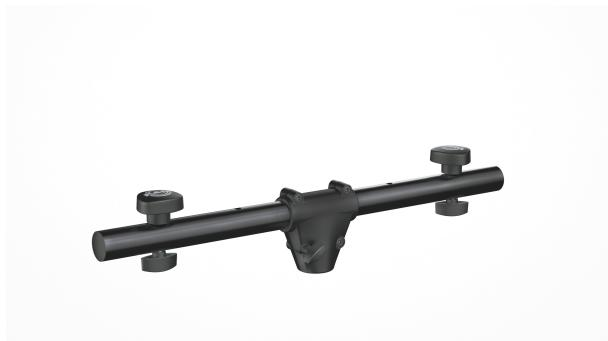
The flexible crossbar made of powder-coated steel has four holes for mounting spotlights and can be mounted either centrally above the 1.38" extension tube or on the side. While the central version can hold up to 55.12 lbs, the side mounting is limited to a load of 22.05 lbs. Two screw sets are included for secure and quick spotlight mounting.
