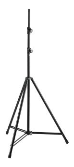
Extending to over 157", this lighting stand is for professional use. The new zinc die-cast clamps and the larger steel leg tubing give this top of the range stand more stability. The infinitely variable non-marring height adjustment can be reinforced with two safety rings. A variety of crossbars may be attached using the M10 thread adaptor.
