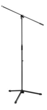
Entry-level, low-priced microphone stand. The practical swivel joint allows the one-piece boom arm to be simultaneously positioned for tilt and length. Thanks to a low weight of only 4.053 lbs, it is particularly suitable for the mobile musician. The stand requires little space as its base diameter is only 25.984". The large foot end caps help to make the stand stable and reduce unpleasant transmission noise.
