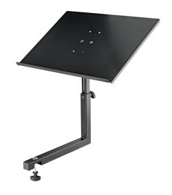
This tray is an extension for the DJ table 12160. With the tray, you get a second level and can thus place additional equipment within reach. The height-adjustable and tiltable plate has a support surface of 15.748 x 11.811" and an integrated stop bar. The inclination can be adjusted from 0 to 32° in 8 steps. Three different positions are available for mounting on the DJ table 12160.
