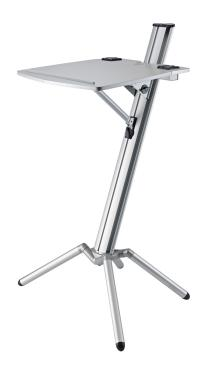
Sturdy, sloping extruded aluminum column, with raised legs (for plenty of leg room). Elegant manuscript rest with an embossed aluminum surface and stop rail. Height and angle are infinitely adjustable. Elegant cable management with feed-through bushing and cable clips. Two 3-pin XLR microphone sockets, acoustically insulated for recording with gooseneck or other lightweight microphones with XLR plugs (not included).
