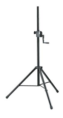
A high quality steel speaker stand with plastic clamps for professional use. Infinitely variable height adjustment with a hand crank and push button system which prevents an uncontrolled reverse motion. There is an additional locking screw for extra safety. Extension tube diameter 1.378", suitable for speakers and lighting crossbars with an integrated M10 thread connector.
