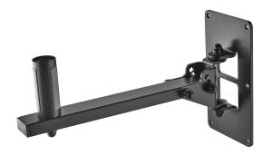
Robust wall mount for holding speakers with flange socket up to 55.115 lbs. The swivel range is continuously adjustable up to 120°. The tilt can be fixed in three steps with 0°, -12.5° and -25°. A patented expanding mandrel ensures a wobble- and vibration-free fit of the speaker. The solid steel construction and durable powder coating ensure long-lasting use.
