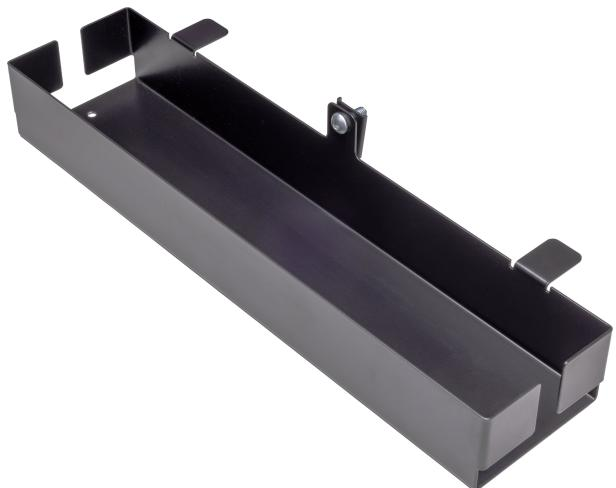
The practical box is attached to the crossbar of the confidence monitor stand close to the ground and is used to hold power strips and neatly store extra-long cables. The solid construction made of sturdy sheet steel has side openings that provide enough space for convenient cable routing. The dimensions are 17.205 x 3.937 x 2.362".
